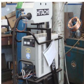
Welder MIG-MAG Hitachi 350A
